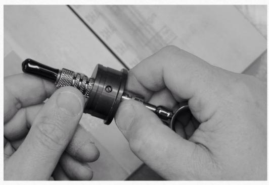
The snap-in bushing uses a spring-loaded indexing pin to hold the swivel knife in place for sharpening. This allows the knife to be quickly loaded into the sharpener.
