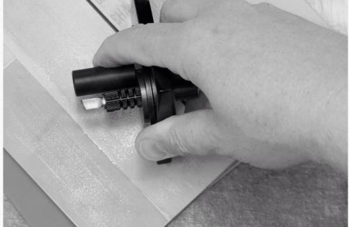
Twist the knife, locking it at the correct distance.
