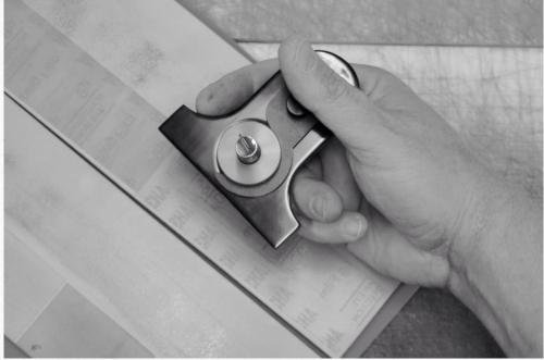
You are now ready to sharpen by tilting the knife blade onto the sharpening medium. Here we are using abrasive film stuck down to a laminate topped Masonite sharpening board which is placed on a urethane mat to hold it in place.
