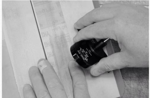
Twist the knife back to the long barrel groove and pull it out to remove it. Strop the blade and go to work.
