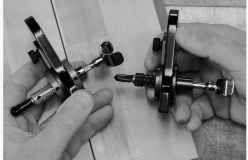
This is the hand piece with a double set screw bushing installed. The bushing and knife are 7/16".
