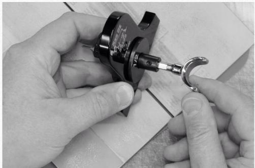
These pictures show the two grips to use. The sharpener is at an angle because an angle blade is being sharpened. This way the blade is kept in-line when sharpened and polished.
