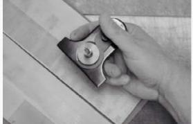
You are now ready to sharpen by tilting the knife blade onto the sharpening medium. Here we are using abrasive film stuck down to a laminate topped Masonite sharpening board which is placed on a urethane mat to hold it in place.
