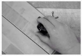
Work through the progressively finer grits until you have polished the blade. Here we see a 3 micron film being used. The blade is finished with 1 micron film, leaving a mirror polish.
