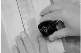
Twist the knife back to the long barrel groove and pull it out to remove it. Strop the blade and go to work.
