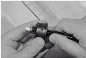
We want the blade to protrude as close to  $1 \frac{1}{2}$  as possible, which will give a bevel angle within half a degree or so of 30 degrees.
