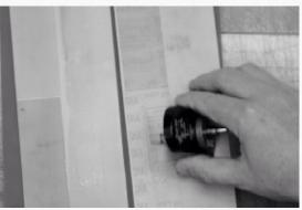
This alternate grip allows you to place a thumb on the blade as you sharpen. Use care not to press more on one side of the blade than the other, **unless** you are working to correct previously off balance sharpening. Use light pressure and let the grit do the work.
