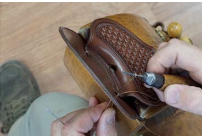
Pulling loop through to the right side.
