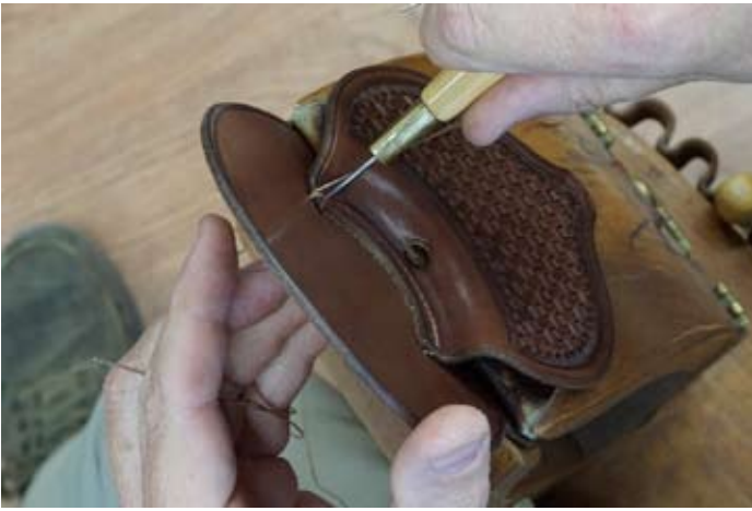
Round awl in use opening the hole.
