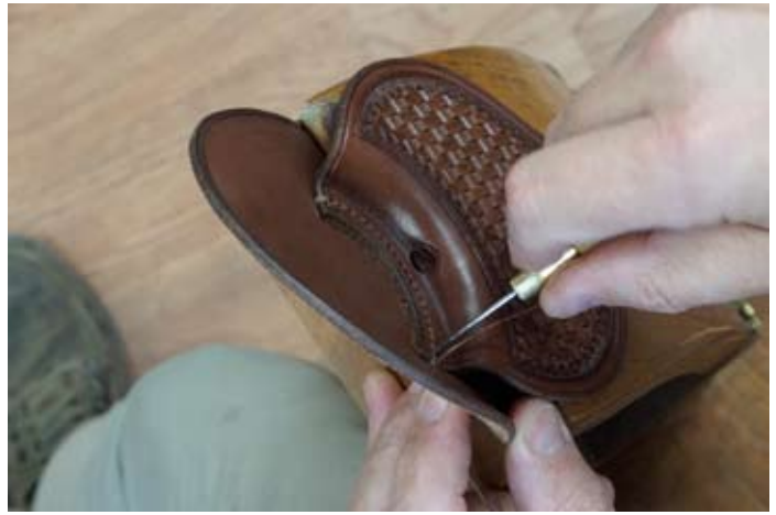
Round awl used to open back stitch.
